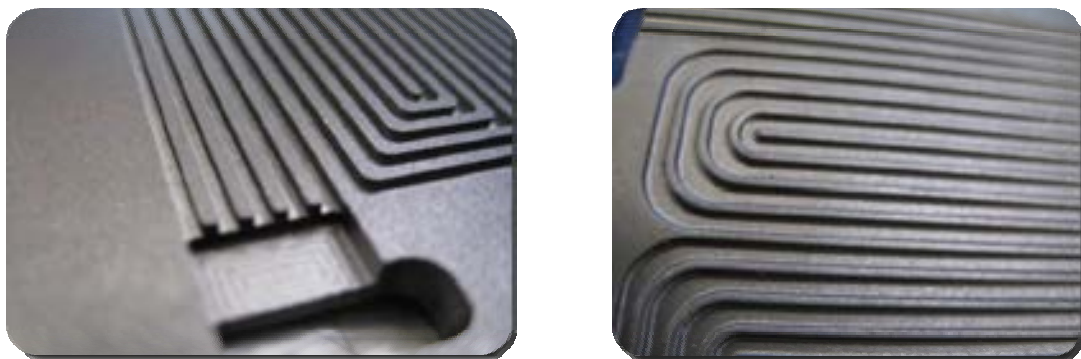
Figure 1.1 & 1.2 Machined and moulded ElectroPhen ® -based bipolar composite plates, respectively
